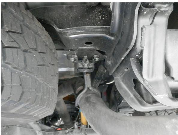
**Step 1.** To remove the OEM system, begin by unclamping the Extension Pipe from the junction behind the DPF. You can then disengage the welded hangers from the rubber insulators and remove the system. Do not damage or discard the rubber insulator it will be reused to mount the new system.
