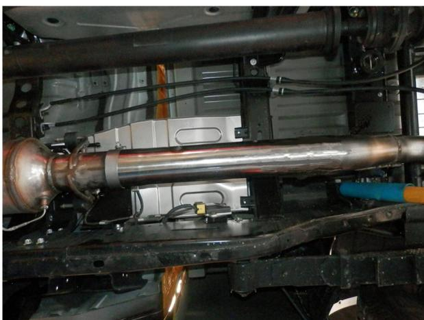
**Step 2.** Begin installation of the Magnaflow system by locating the indexing notch to the OEM peg then loosely clamping the Inlet Pipe Assembly to the outlet of the DPF using a supplied 4.00" clamp.
