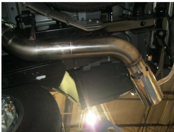
**Step 3.** Finish by loosely installing the Tail Pipe Assembly to the Inlet Pipe Assembly using a supplied 5.00" clamp and fitting the welded hanger into the rubber insulator.
