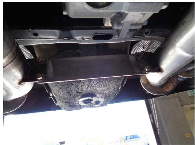
Step 3: Next Install the Muffler Assemblies to the outlets of the Resonator Assembly using the supplied 2.50" clamps. Insert hangers into rubber insulators. At this time loosely attach the Magnaflow logo brace to tie the muffler assemblies together using the supplied fasteners.
