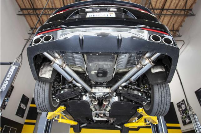
Step 4: Once a final position has been chosen for the new exhaust system, evenly tighten all clamps from front to rear using the torque specifications on page one of these instructions. Tighten fasteners for Muffler brace and install factory underbody brace. Inspect all fasteners after 25-50 miles for operation and re-tighten if necessary.
