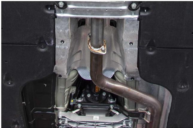
Step 1. To extract the OEM exhaust system you will first need to remove the brace located in front of the factory resonator. Next un-fasten the flanges located behind the catalytic converters and resonator and disengage all welded hangers from the rubber insulators. Do not damage or discard the rubber insulators or fasteners as they will be re-used to mount the new system. You can now remove the exhaust from the vehicle.
