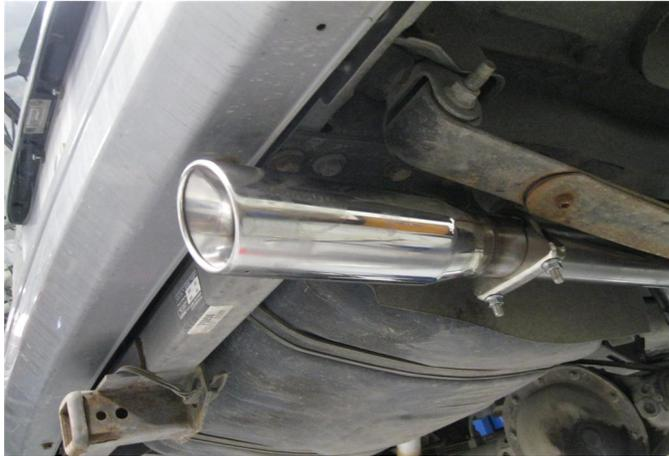
**Step 4.** Loosely secure the tip section of the Tail Pipe Assembly to the OEM hanger using the supplied 2.50" U-Bolt clamp.
