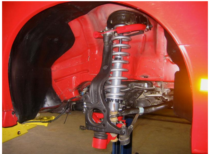
Image 4- Upper and Lower A-Arms installed.
